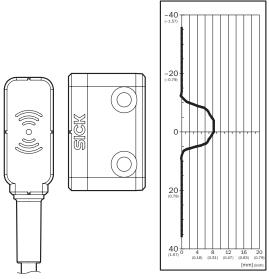
Safe switch on distance  $S_{ao}\,6\,\text{mm}$
