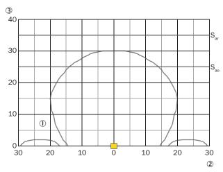
If the actuator moves laterally in relation to the surface of the sensor, a minimum distance of 3 mm must be maintained. This distance will prevent premature triggering due to the side approach areas.
