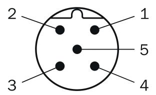
Connector M12, 5-pin, A-coded
