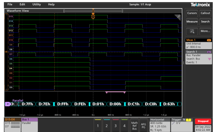
Digital channel trigger and decode
