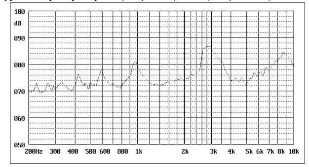
Typical Frequency Response (3.6V0-p sine-sweep with microphone spaced at 10cm)
