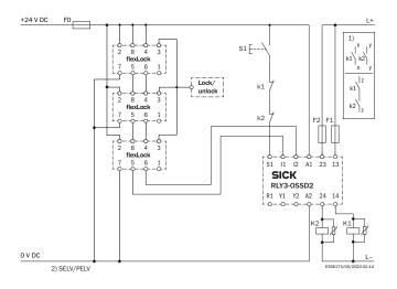
flexLock safety locking device to RLY3-OSSD2 safety relay
