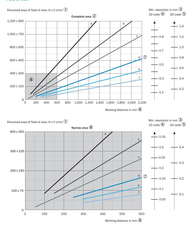
For S-mount and standard C-mount lenses, spacer rings are needed for working distances shorter than approximately 10 times the focal length. For compact C-mount lenses, spacer rings are not needed, but the built-in illumination cannot be used for distances shorter than 300 mm.
