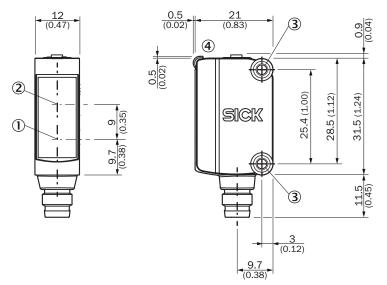
① Center of optical axis, sender
