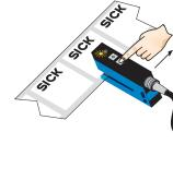
Press both the "+" and "-" buttons together, hold > 1 s and than release the teach-in buttons. The red LED flashes.
