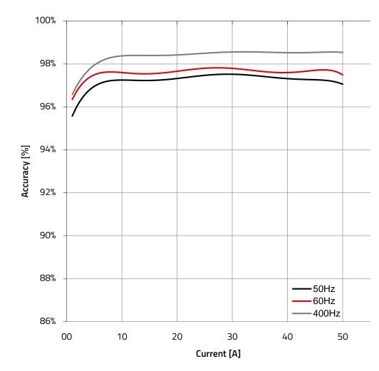
Response testing was completed with a burden resistor value of  $11.11\Omega$  to achieve a 1V output at 45A.
