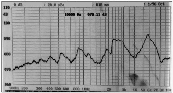
Typical Frequency Response (5 V0-p sine-sweep with microphone spaced at 10cm)
