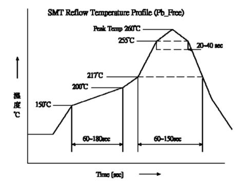
\*Manual Solder - Iron Temp 350C and solder time 2-3sec per terminal.
