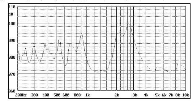
Typical Frequency Response (12Vp-p sine-sweep with microphone spaced at 10cm)
