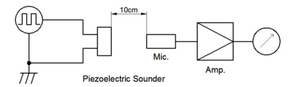
MIC: ND10 Sound Meter or equivalent Signal Generator: DF1641D or equivalent
