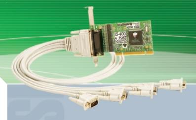
This card provides 4 industry standard RS232 serial COM ports in a single PCI slot. A fully moulded quad cable terminated in 9 pin male D plug ensures a reliable connection.
