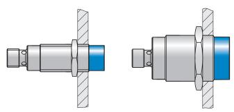
Required overrun of the active cap (blue) when mounting the device in metal (non-flush installation)
