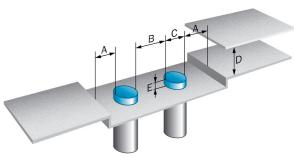
Distances required to prevent mutual interference with parallel mounting of several devices as well as from the environment. RFH505/510 (in metal)
