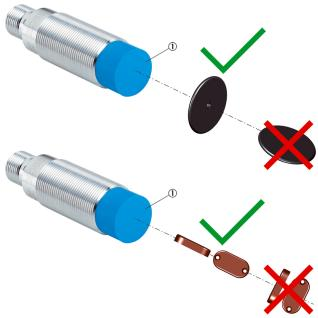
Optimal alignment of the transponders for a reliable read and write process  ${\tt @}$  Cap with integrated antenna
