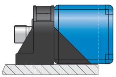
Recommended overrun of the active head when mounting the device on metal: about 10 mm
