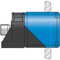
Recommended overrun of the active head when mounting the device in metal: about 10 mm (non-flush installation) RFH515 (on metal)
