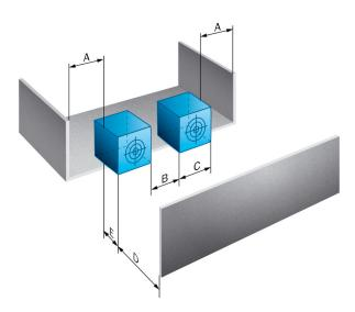
Distances required to prevent mutual interference with parallel mounting of several devices as well as from the environment. RFH515 (in metal)
