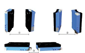
Distances required to prevent mutual interference with mounting of two devices.
