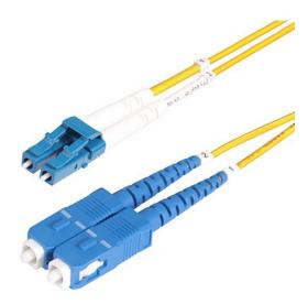
OS2 LC to SC Single Mode Duplex Fiber Optic Patch cable facilitates connectivity across 100G networks. It supports Coarse Wavelength Division Multiplexing (CWDM) across an extended wavelength range of 1260-1625nm, improving channel isolation for optimal signal strength over long distances.
