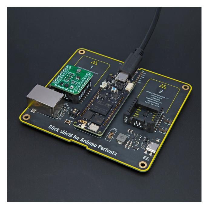
When the USB is connected to the Portenta board, the PWR diode will glow Green, and at this setup, the Portenta H7 baseboard itself will be supplied, and it will provide power to the Click Shield, including all mikroBUS<sup>™</sup> sockets.
