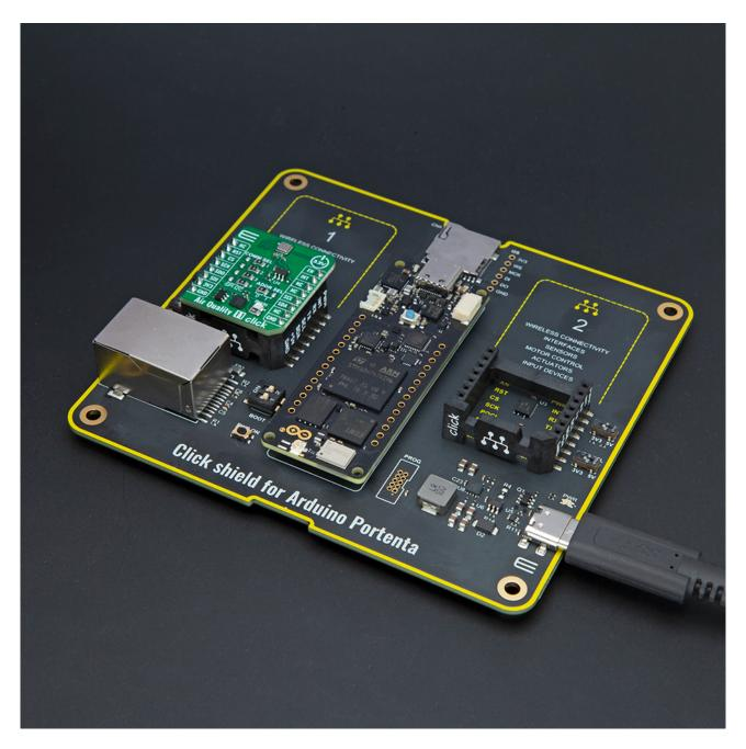
When the USB is connected to the Click Shield, the PWR diode will glow Blue, and at this setup, the connected Portenta baseboard and all mikroBUS<sup>™</sup> sockets will be powered from it.
