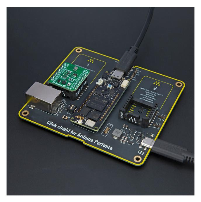
When the USB is connected to the Click Shield, and the other USB is connected to the Portenta board, the PWR diode will glow Cyan, and at this setup, the mikroBUS<sup>™</sup> sockets are powered from the Type C connector from Click Shield.
