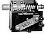
AC Series Door Switch, Single Pole Double Throw Circuitry, 15 A at 250 Vac, Rod Actuator, Silver Contacts, Screw Termination
