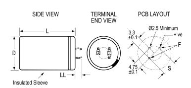
General Information Series ALA8A Dielectric Aluminum Electrolytic Description Snap-In, Aluminum Electrolytic RoHS Lead 3 Pin Short Qualifications AEC-Q200 AEC-Q200 Yes Halogen Free Yes Typical Component Weight 30 g Shelf Life 156 Weeks
