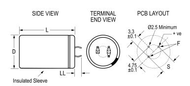
General Information Series ALA8A Dielectric Aluminum Electrolytic Description Snap-In, Aluminum Electrolytic RoHS Lead 3 Pin Short Qualifications AEC-Q200 AEC-Q200 Yes Halogen Free Yes Typical Component Weight 45 g Shelf Life 156 Weeks
