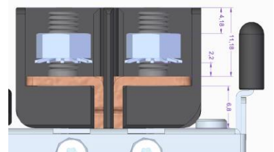
Figure 25. Height of fixed screw (Unit: mm)
