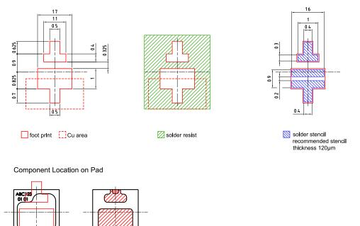
For superior solder joint connectivity results we recommend soldering under standard nitrogen atmosphere.
