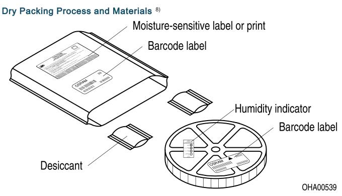
Moisture-sensitive product is packed in a dry bag containing desiccant and a humidity card according JEDEC-STD-033.
