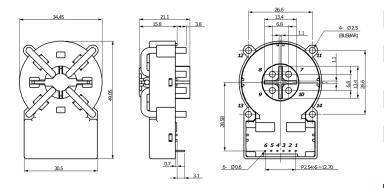
General Information Series FG-R02 Type Current Style Through-Hole Description Fluxgate-Based Residual Current Sensor Open-loop, Fluxgate-Based Current Detection, PCB Features Mounting Lead 6 Pin RoHS Yes **REACH** Yes Qualifications **IEC**
