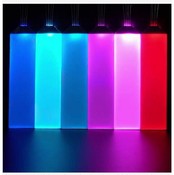
The RGB LCD backlight panel uses the RGB color model, this is an industry color standard that produces a wide variety of colors by varying three color channels: red (R), green (G), and blue (B), a total of 16 million colors, nearly all colors that human vision can perceive.
