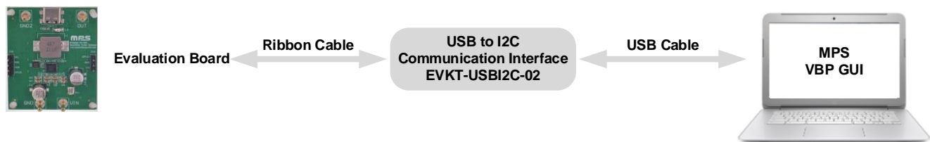
Figure 1: EVKT-MPQ4242 Evaluation Kit Set-Up
