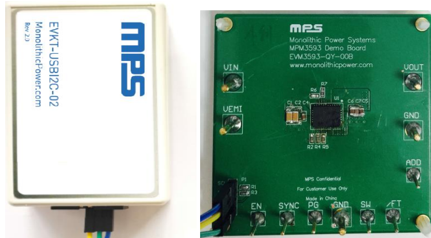
Figure 5: EVB to MPS I 2 C Communication Interface Device Wire Connection
