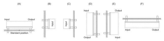
■Option-N model can be mounted in the mounting position shown in the figure below. The installation of (F) possible only forced air cooling.
