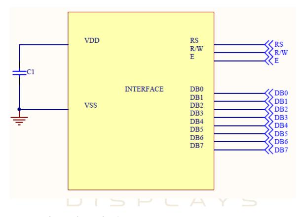
Pin connected to MCU interface: RS, R/W, E, DB0~DB7
