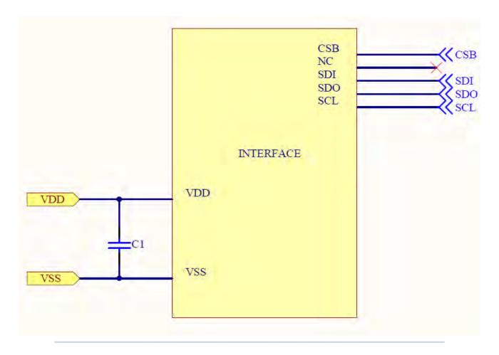
Pin connected to MCU interface: CSB, SDI,SDO, SCLURE • SUPPLY
