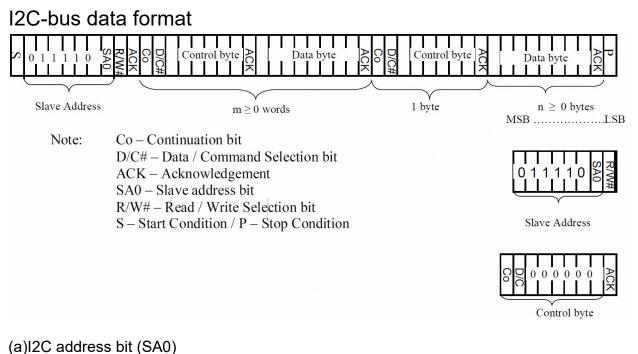
The slave address is following the start condition for recognition use. The slave address is either "b0111100" or "b0111101" by changing the SA0 to LOW or HIGH (D/C pin acts as SA0).
