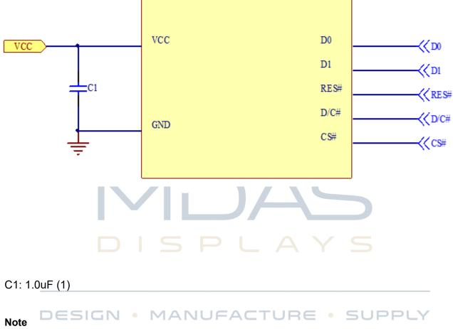
(1) The capacitor value is recommended value. Select appropriate value against module application.
