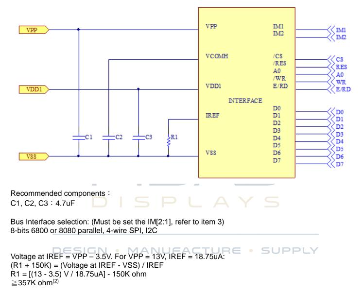
R1 recommends 562K ohm. If new module want to be compatible with hardware using past module (IC SSD1309 with higher R1), then the initial code must be modified to meet typical brightness (adjust contrast or VCOM to higher level).
