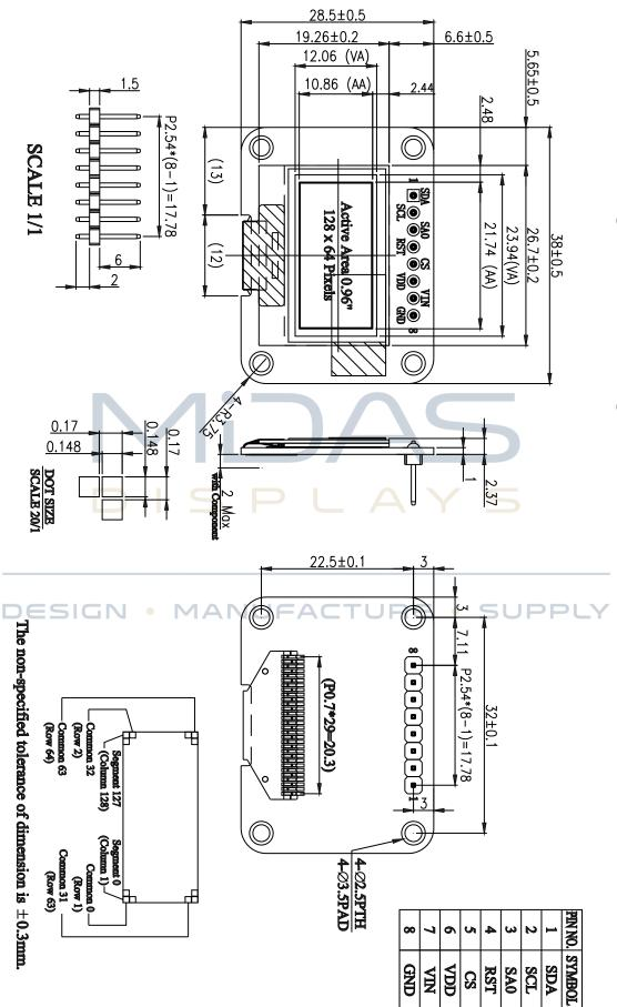
**Contour Drawing & Block Diagram**
