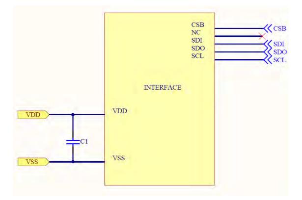
Recommended components : MANUFACTURE • SUPPLY C1 : 1.0uF
