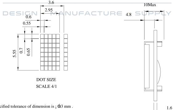
The non-specified tolerance of dimension is ;  $\hat{\mathbf{0}}3 \text{ mm}$ .
