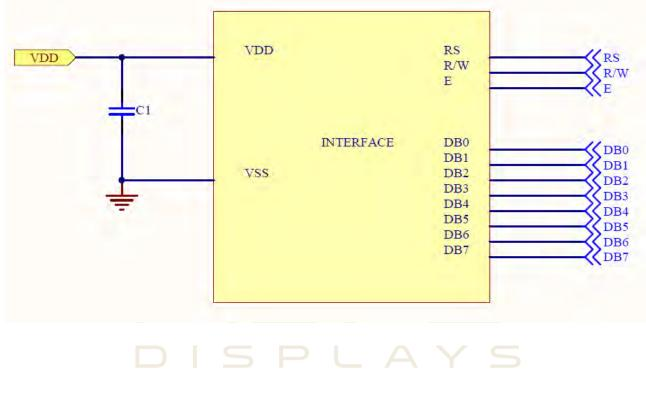
Pin connected to MCU interface: RS, R/W, E, DB0~7
