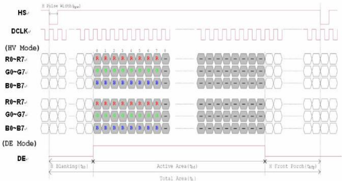
Figure 3. 1 Horizontal input timing diagram.
