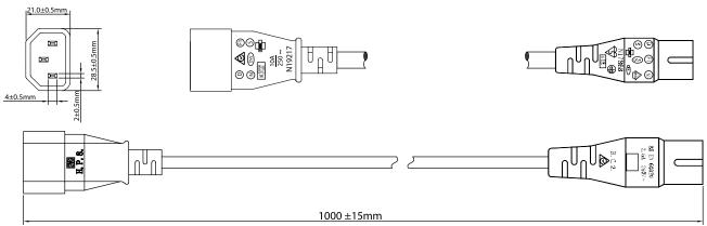
CABLE MARKING:H03VVH2-F 2X0.75mm² ⊲VDE⊳ N19626 60227 IEC 52 300/300V CABLE COLOUR: BLACK
