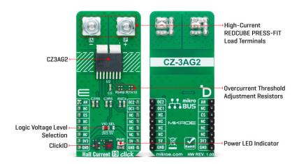
As mentioned, this Click board<sup>™</sup> is equipped with dual overcurrent detection capabilities on the OC1 and OC2 pins of the mikroBUS™ socket. Using voltage dividers R6/R9 and R7/R10, it sets precise current limits ranging from 7A to 17.5A. This ensures that any current value falling outside this specified range will be promptly detected by the overcurrent detectors, providing reliable protection and accurate measurement.
