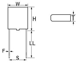
**General Information** Series T340 Dielectric MnO2 Tantalum Style Radial Molded Description Radial, Solid Tantalum, Molded RoHS Yes Termination Tin AEC-Q200 No Construction Molded Includes Standoff Height of 0.38 +/- 0.13mm. Miscellaneous Longest Lead Is Positive. Notes
