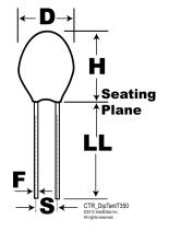
**General Information** Series T350 Dielectric MnO2 Tantalum Style Radial Radial, Solid Tantalum, Conformal, Dipped Description Features Low Leakage RoHS Yes Termination Tin AEC-Q200 No Notes Longest Lead Is Positive.
