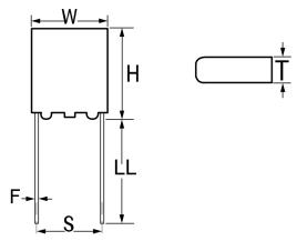
Series T340 Dielectric MnO2 Tantalum Style Radial Molded Description Radial, Solid Tantalum, Molded RoHS Yes Termination Tin AEC-Q200 No Construction Molded Includes Standoff Height of 0.38 +/- 0.13mm. Miscellaneous Longest Lead Is Positive. Notes
