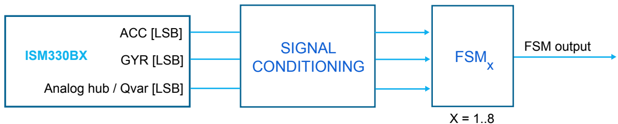
Figure 2. State machine in the ISM330BX
