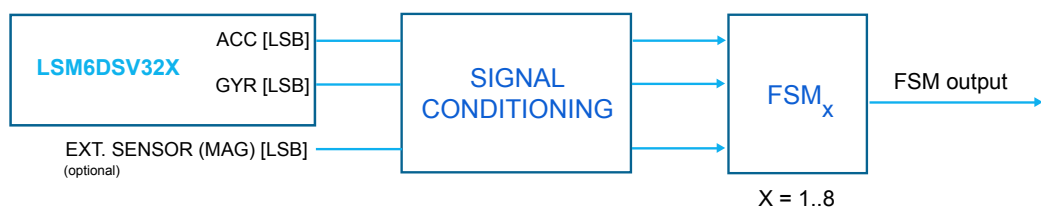
Figure 3. State machine in the LSM6DSV32X
