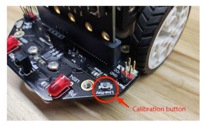
1.Place the car in the black area of the map that comes with the product, and make sure the left and right sides of the sensor are in the area, as shown in the picture below:
