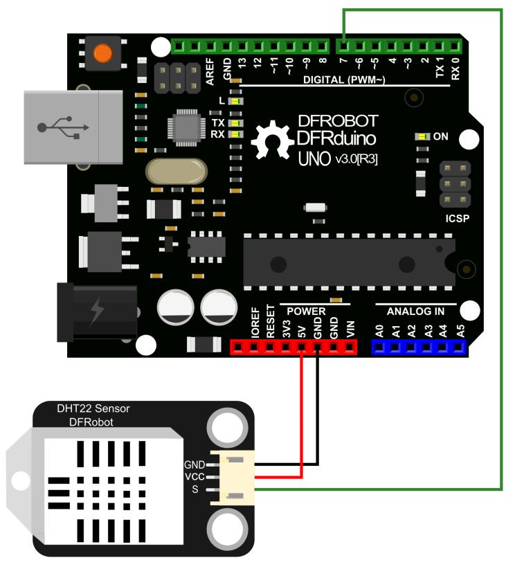
Please download the Library of DHT22 (https://github.com/CainZ/DHT) at first. This program is used to test the temperature and humidity of the DHT22
