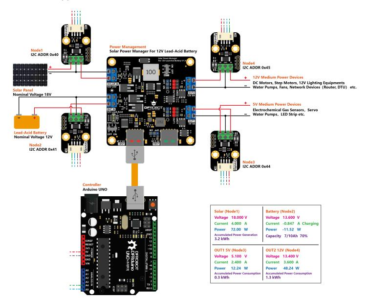
Note: Since most solar management modules have battery protection that disconnects GND from BAT-. If you connect BAT- to GND as shown in the above diagram to monitor the battery level, it will result in BAT- not being able to disconnect GND and disable the battery protection circuit of the solar management
