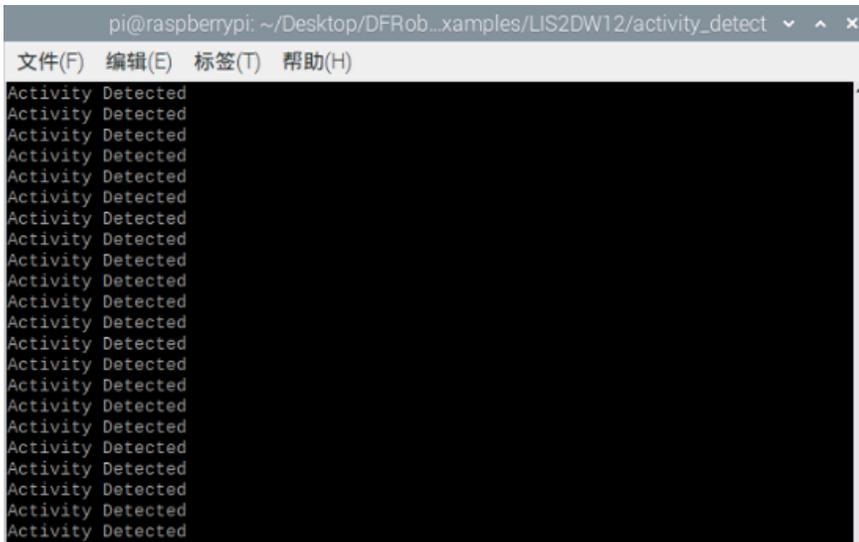
A terminal window screenshot showing the output of the 'activity\_detect.py' script. The window title is 'pi@raspberrypi: ~/Desktop/DFRob...amples/LIS2DW12/activity\_detect'. The menu bar includes '文件(F)', '编辑(E)', '标签(T)', and '帮助(H)'. The terminal output consists of 20 lines, each displaying 'Activity Detected'.
