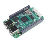
IoT made easy with WiFi/Bluetooth and a variety of sensors attached with Grove Connectors from SeeedStudio using this differentiated version of the open-source BeagleBone® Black hardware design
