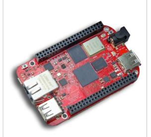
Supporting an extended temperature range, upgraded Ethernet, wireless and extra USB port capability, the SanCloud BeagleBone® Enhanced Extended WiFi brings the extras you need for IIoT applications
